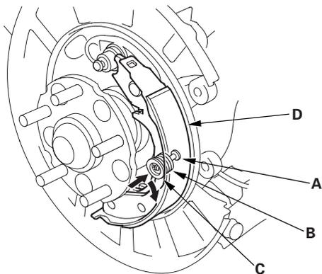
6. Clean the threaded portions of the clevis A, and coat the threads with multipurpose grease. Clean the sliding surface of the clevis B, and coat the sliding surface with multipurpose grease. Install the clevis A and B on the adjuster (C), and shorten the clevis A by turning the adjuster.
