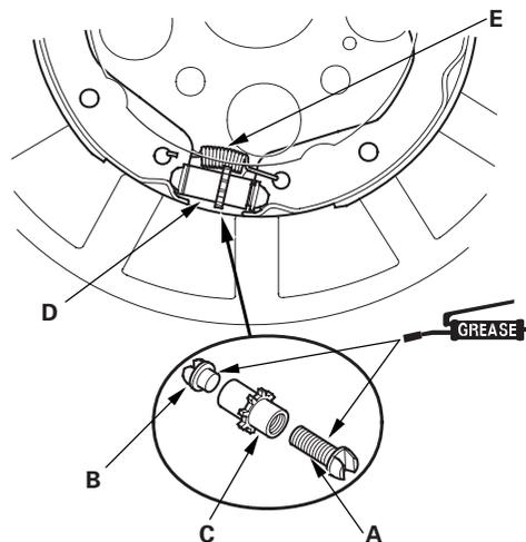
7. Reinstall the brake shoe adjuster assembly (D), and hook the lower return spring (E) on the parking brake shoes.
